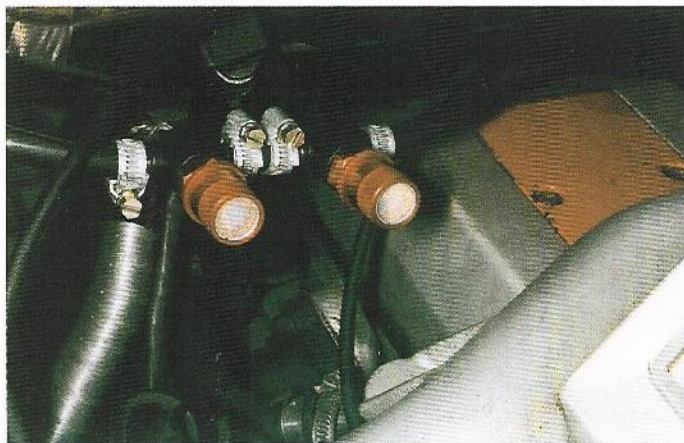
As this Senator has a 3.0-litre engine, two separate Ecotek units are required. For cars up to 2.6 litres in capacity, one is enough
