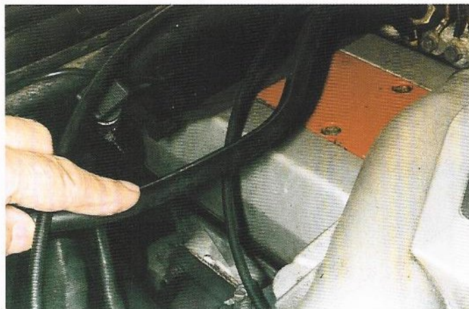
On this Vauxhall Senator, proper fitting involved cutting this tube and reconnecting it carefully afterwards
